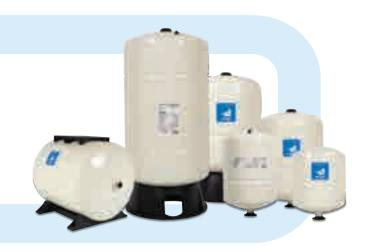
The PressureWave<sup>TM</sup> series is constructed of a virgin polypropylene liner combined with an FDA compliant high-grade butyl diaphragm. This is held against the wall of the tank with a steel clench ring. The brass air valve, sealed by a threaded O-ring valve cap, prevents air leaks. Water enters the tank through a patented stainless-steel water connection.
