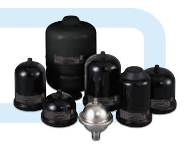
HydroGuard™ shock arrestors are specially built with the latest diaphragm technology designed to reduce and eliminate hydraulic shock. The internal diaphragm divides the arrestor into separate air and water chambers. The sealed air chamber acts as a cushion that compresses when the water pressure suddenly increases or surges due to hydraulic shock.
